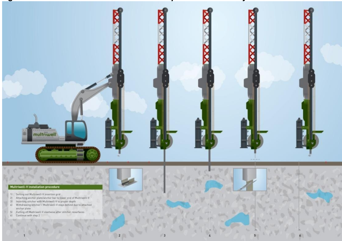
Figure 3-4 Overview installation vertical part of Multiwell system
